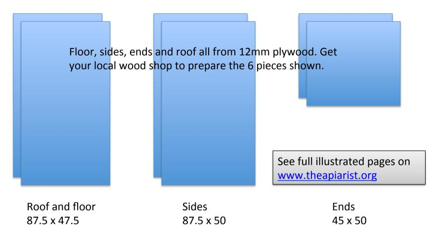
**Also required** – 2 x 40x5x3 and 2 x 30x5x3 softwood (feet and handles, sizes not critical). 30-40mm screws, wood glue, contact adhesive, strong tape. 5 x 100x50x5 insulation (Jablight). Scrap wood. Ecostat heating element.
